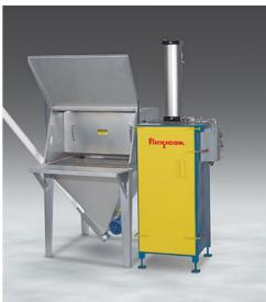
Dust generated from bag dumping and compaction is drawn onto cartridge filters equipped with air nozzles that cause collected dust to fall into the hopper on a timed cycle, conserving useable material while protecting plant personnel. An enclosed flexible screw conveyor transports material at any angle.
